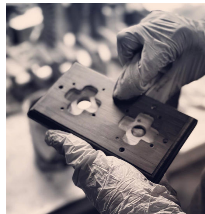
◀◀ Hand finishing a wooden pattress in our UK workshop for a Double Period Switch
